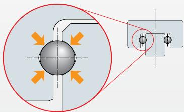
Although small in size, it provides stable accuracy and rigidity due to its simple design, even in operations under fluctuating loads with changing direction and magnitude or complex loads. Standard products are made of stainless steel and a wide range of variations in shapes and sizes are available.
